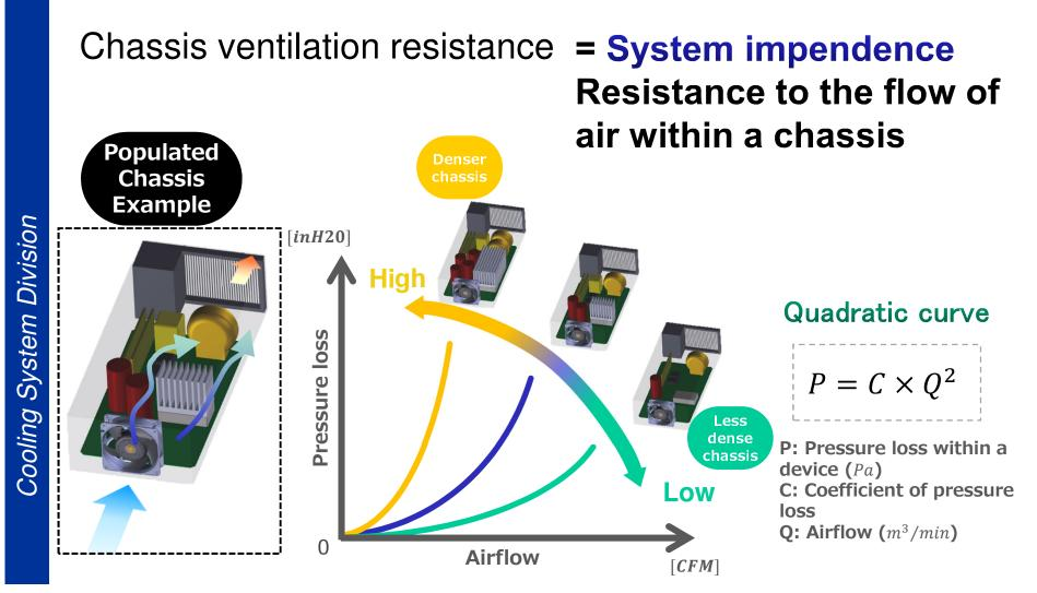
System impedance curves get steeper with denser chassis layout
