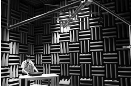
Acoustic radio wave anechoic chamber
