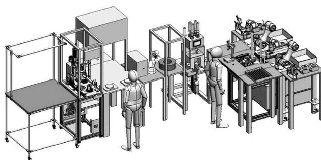
Fig. 7 56 mm sq. stepping motor assembly line
