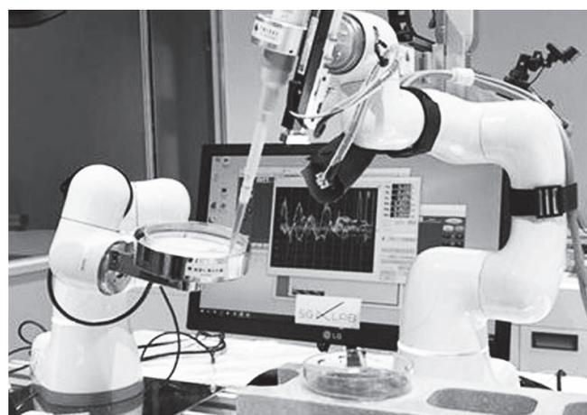
Fig. 5 Pipette operation (remote robot arm side)
