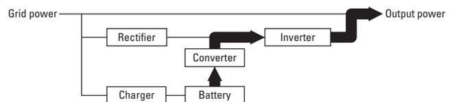
Fig. 5 The power supply path during a power grid failure
