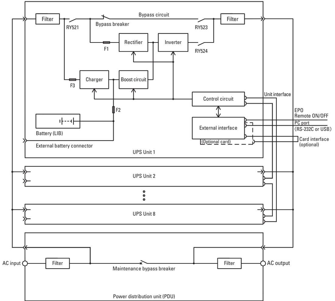
Fig. 6 A11M-Li system diagram
