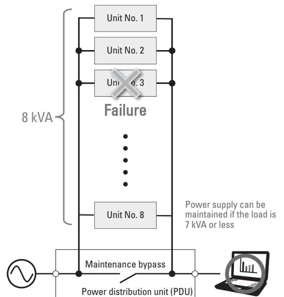
Fig. 7 Parallel redundant operation
