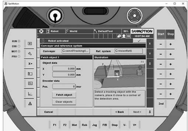
Fig. 11 Belt conveyor and camera setting screen
