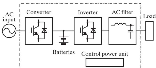
Fig. 1 Example of basic UPS circuit configuration
