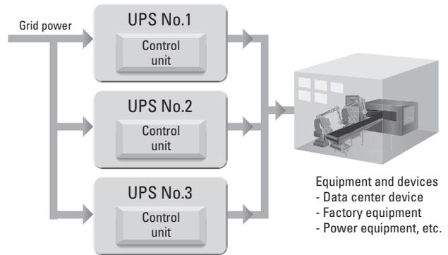
Fig. 7 Fully autonomous control method
