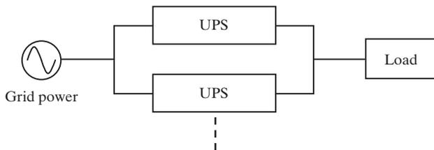
Fig. 6 Parallel redundant operation system diagram
