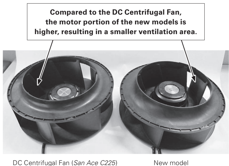
Fig. 7 Comparison of new model and DC Centrifugal Fan impellers
