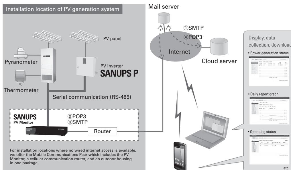
Fig. 3: System configuration
