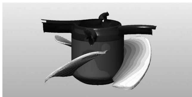
Fig. 1: Example of pressure distribution on the blade surface using fluid analysis
