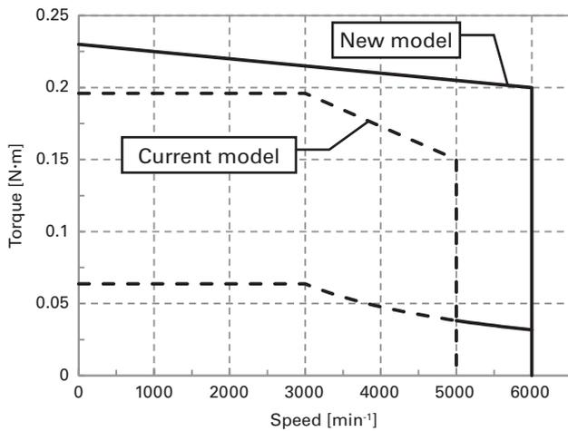
Fig. 3: Torque vs. speed characteristics (SANYO DENKI amplifier combination, 48 VDC)
