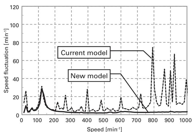
Fig. 1: Comparison of speed fluctuation with the current model
