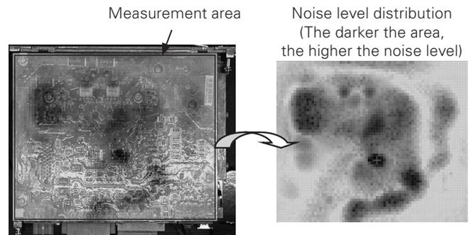
Fig. 4: PCB of a prototype production machine (before countermeasures)
