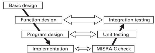
Fig. 6: Software design and testing processes.
