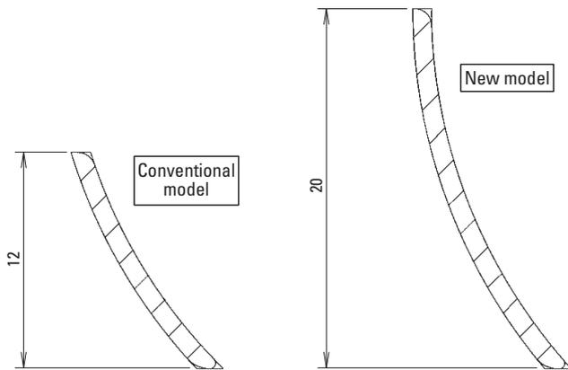
Fig. 4: Static blade cross section comparison
