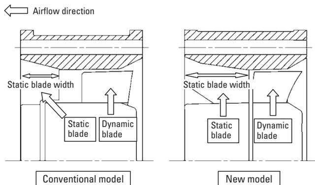
Fig. 5: Structural cross section comparison
