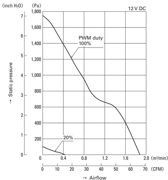
Fig. 3: Airflow - static pressure
