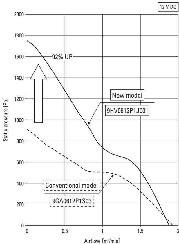
Fig. 7: Airflow – static pressure comparison
