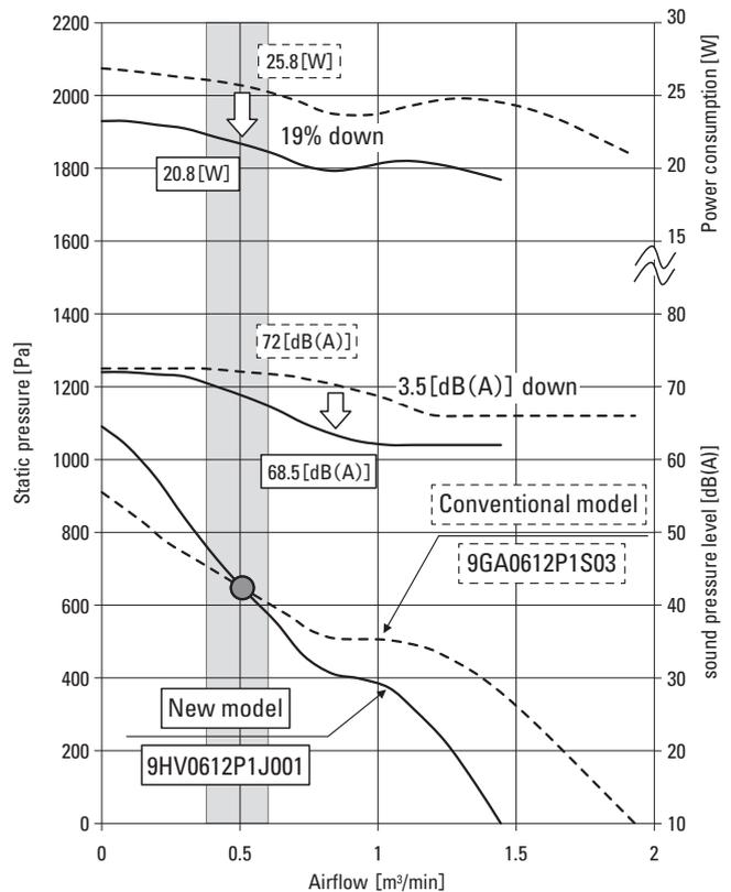
Fig. 8: Airflow – static pressure – SPL – Power comparison
