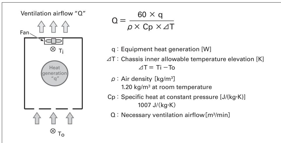
Fig. 6: The amount of heat which should be taken and necessary ventilation
