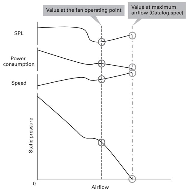
Fig. 4: Operating point and fan characteristic examples
