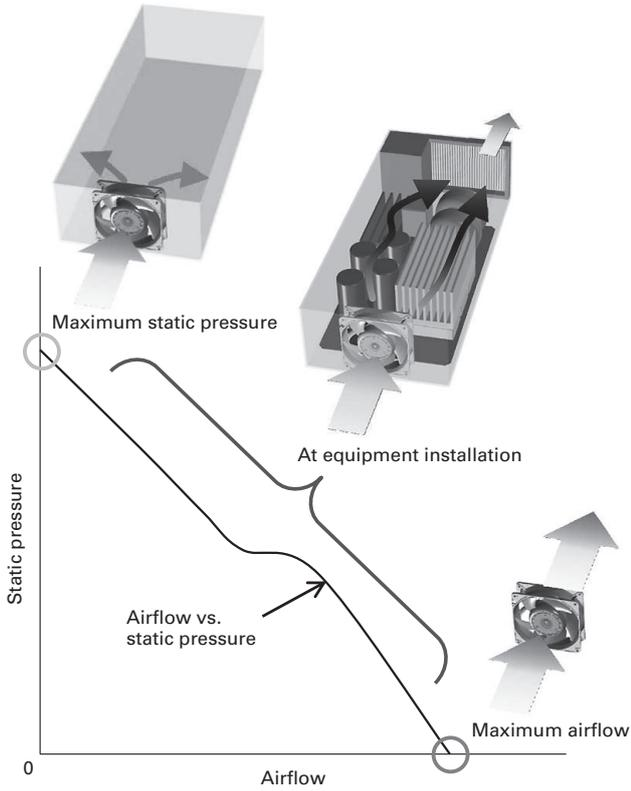
Fig. 2: Airflow vs. static pressure
