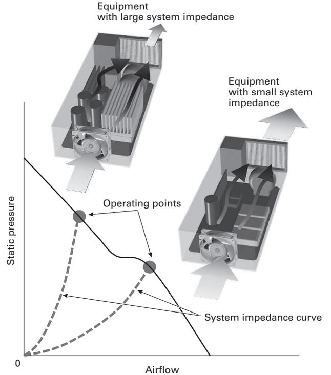
Fig. 3: Airflow vs. static pressure characteristic and system impedance
