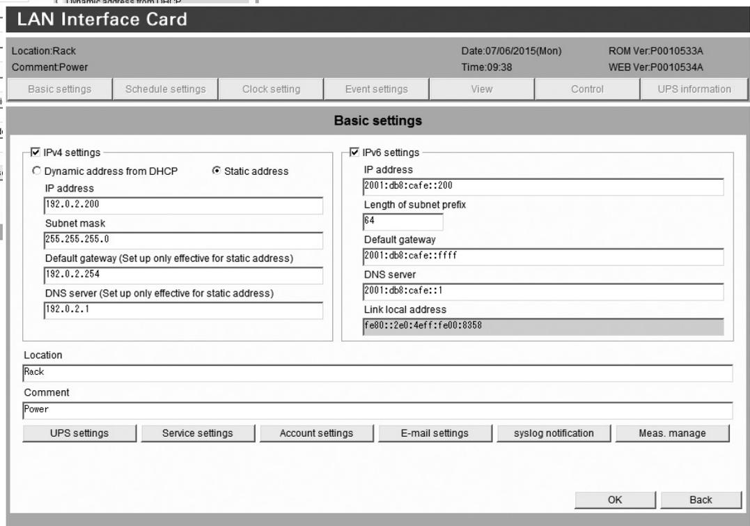
Fig. 3: Setting screen of the new model
