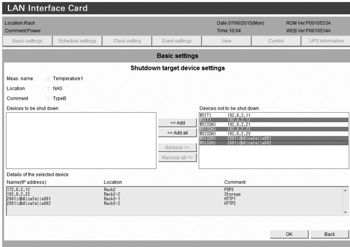
Fig. 4: Screen for selecting devices targeted by sensors
