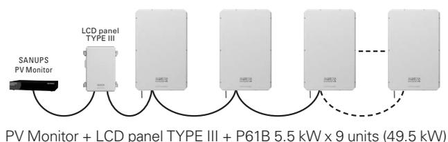
Fig. 2: Main system configuration
