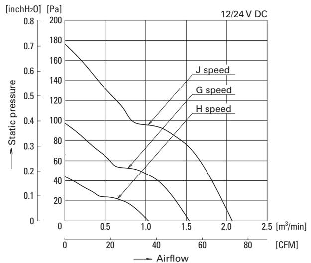
Fig. 6: Airflow vs. static pressure characteristics of "San Ace 80W"
