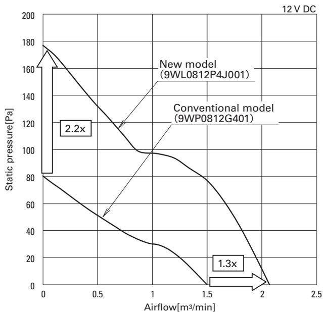
Fig. 9: Airflow vs. static pressure characteristics of "San Ace 80W"
