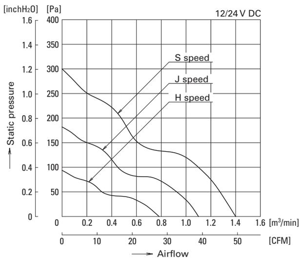
Fig. 5: Airflow vs. static pressure characteristics of "San Ace 60W"
