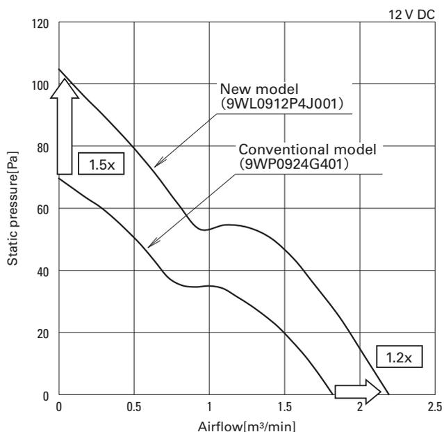
Fig. 10: Airflow vs. static pressure characteristics of "San Ace 92W"
