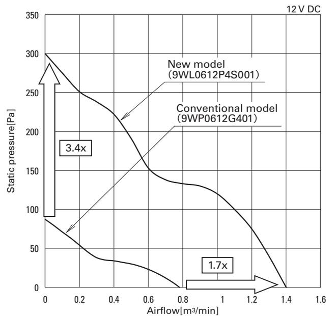
Fig. 8: Airflow vs. static pressure characteristics of "San Ace 60W" New/conventional model comparison
