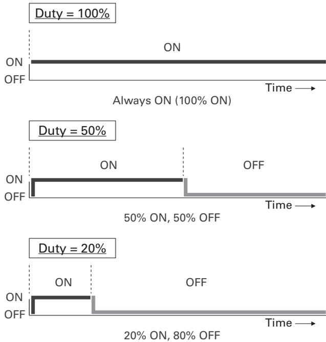
Fig. 5: Example of a PWM control input wave form
