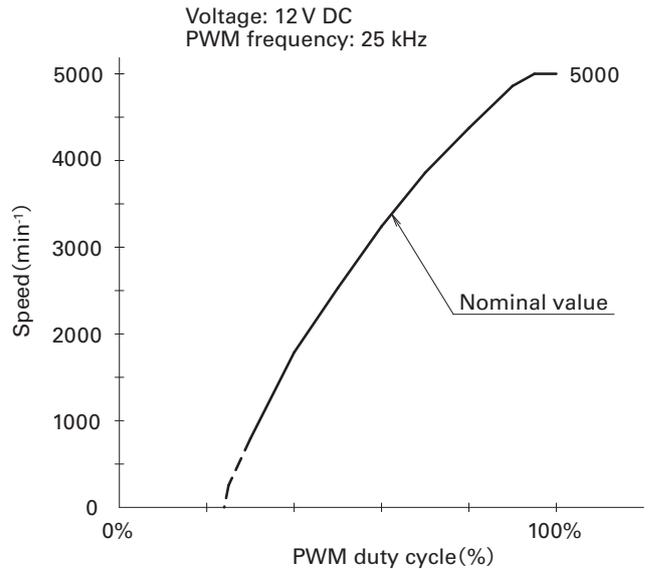
Fig. 6: PWM duty cycle vs. Speed curve Specification for stopping at 0% duty input
