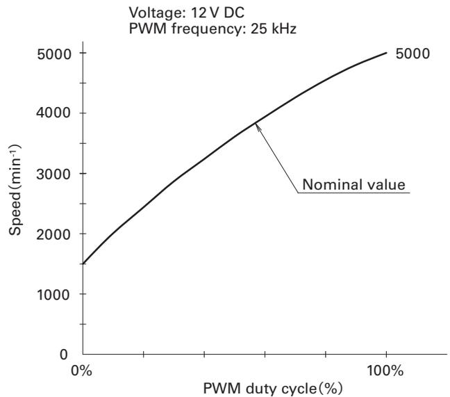
Fig. 7: PWM duty cycle vs. Speed curve Specification for low-speed at 0% duty input
