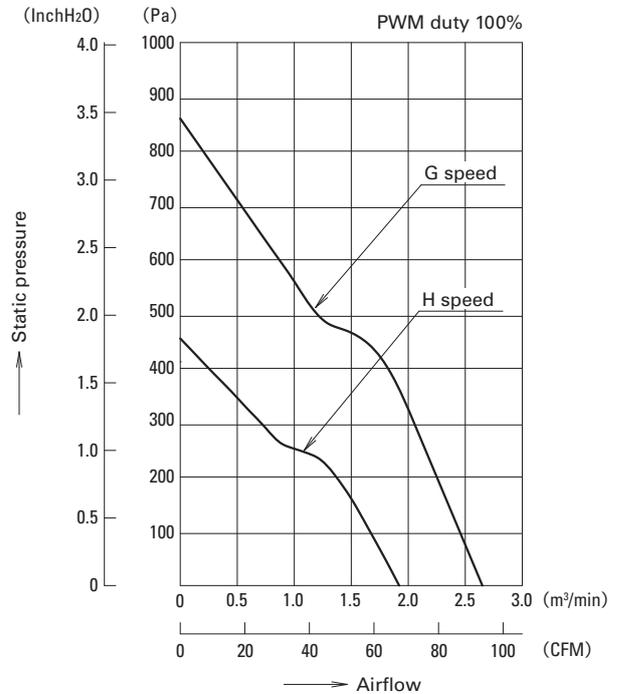
Fig. 3: Airflow vs. static pressure characteristics of the new model
