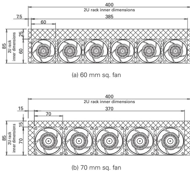
Fig. 6: Installation on a 2U unit
