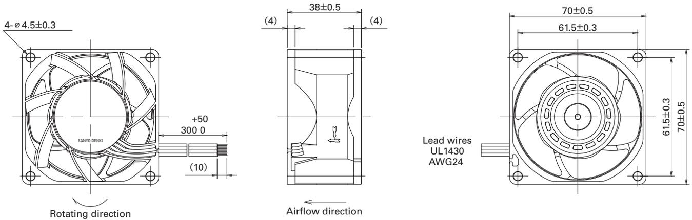
Fig. 2: Dimensions of the new model (unit: mm)
