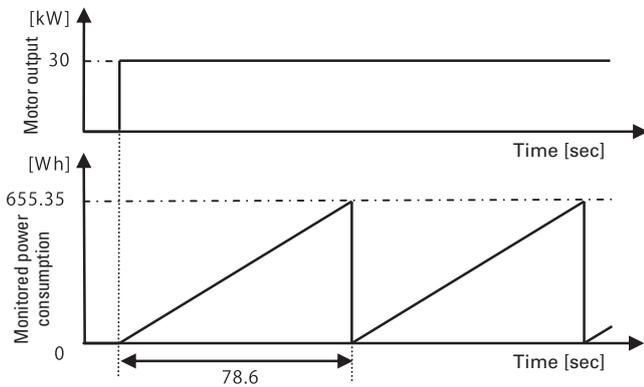
Fig. 6: Image of monitored power consumption output
