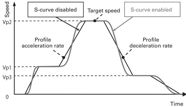
Fig. 8: S-curve motion profile in velocity control
