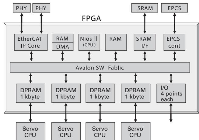
Fig. 5: FPGA configuration for 4-axes communication
