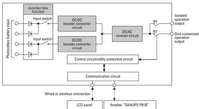
Fig. 4: Circuit block diagram (5 kW model)
