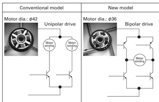
Fig.3: Comparison of size and drive system for conventional model and new model
