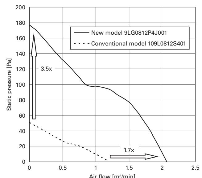
Fig. 2: Comparison of air flow - static pressure characteristics between our conventional model and new model
