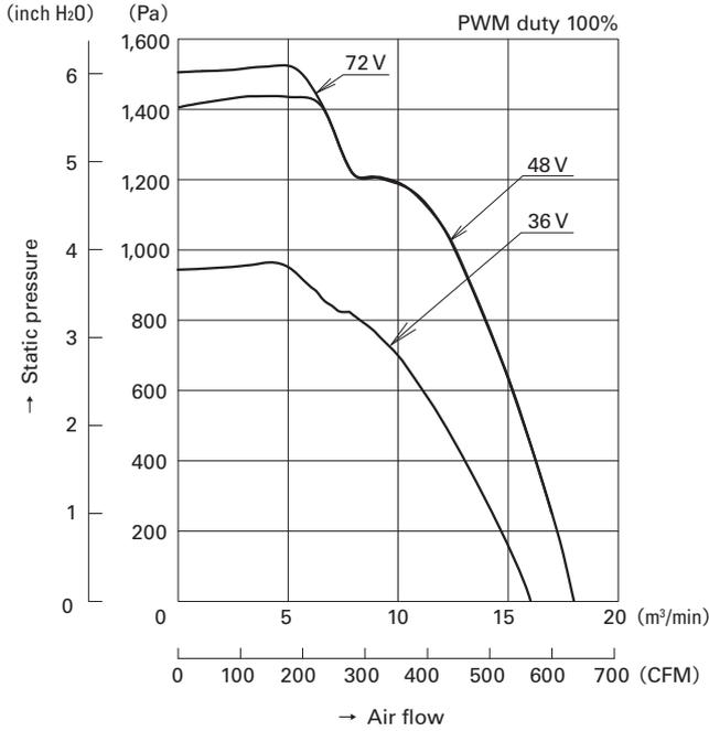
Fig. 3: Air flow vs. static pressure
