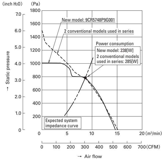
Fig. 6: Example of air flow vs static pressure with the expected system impedance
