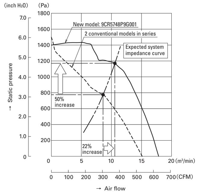
Fig. 5: Air flow vs static pressure characteristics (comparison between the conventional model and the new model)
