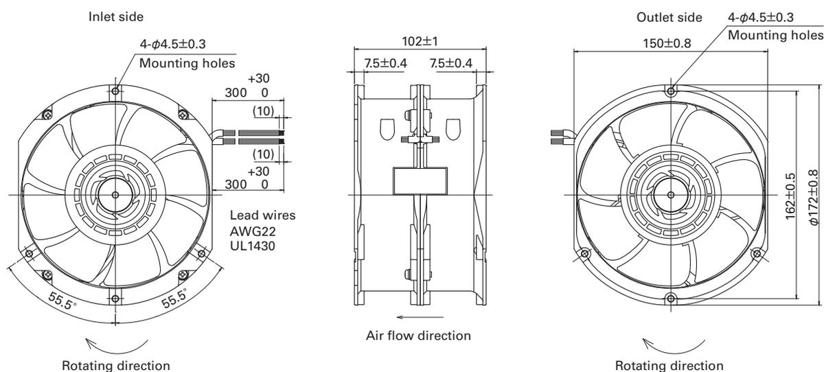
Fig. 2: Dimensions of the new model (unit: mm)
