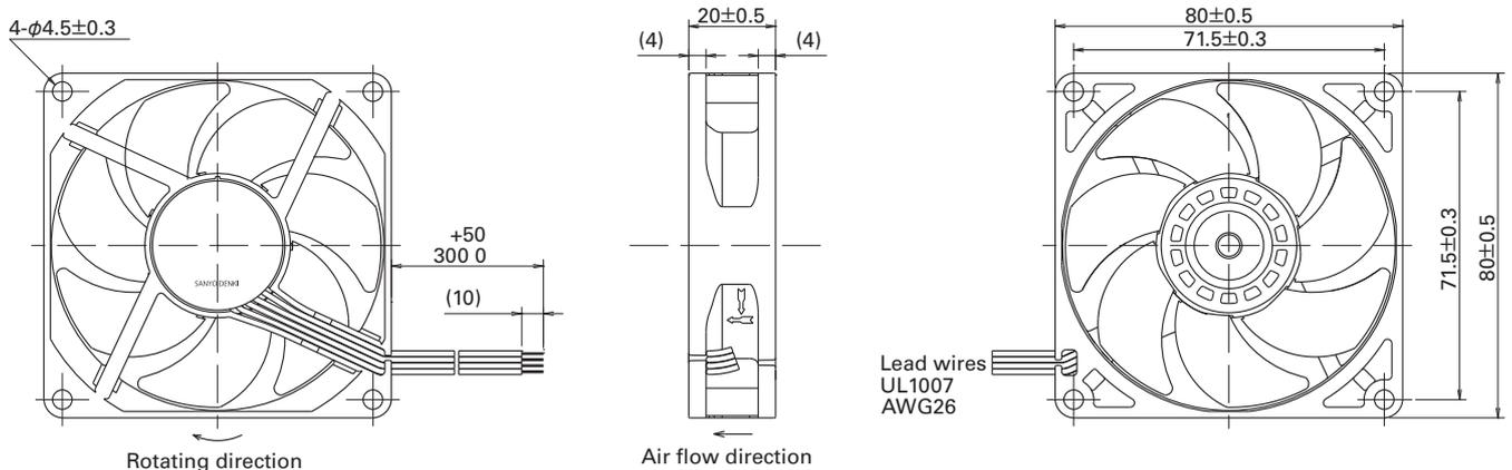
Fig. 2: "San Ace 80" GA type dimensions (unit: mm)
