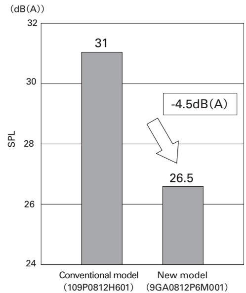
Fig. 8: Comparison of SPL during free air conditions
