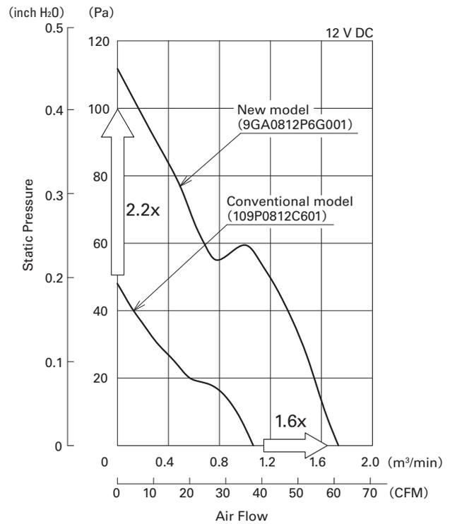
Fig. 5: Air flow vs static pressure characteristics between our conventional model and the new model
