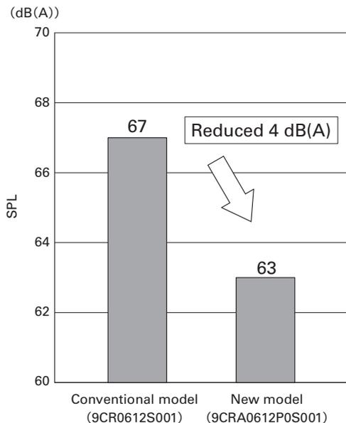
Fig. 10: Comparison of sound pressure level when operated at presumed system impedance
