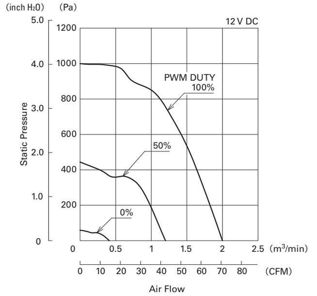
Fig. 5: Air flow vs static pressure characteristics at individual PWM duty cycle(9CRA0612P0G001)
