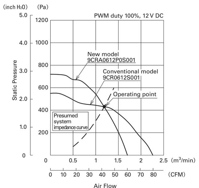
Fig. 8: Air flow vs static pressure characteristics (Comparison between the conventional model and 9CRA0612P0S001)
