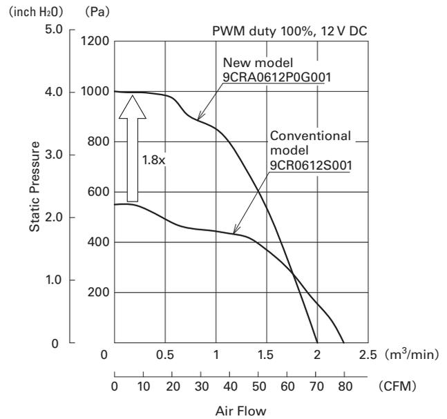
Fig. 7: Air flow vs static pressure characteristics (Comparison between the conventional model and 9CRA0612P0G001)
