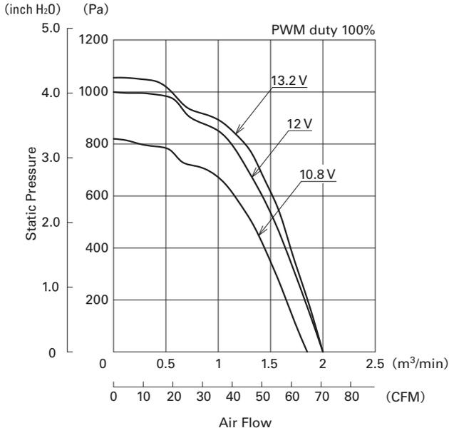
Fig. 3: Air flow vs static pressure characteristics (9CRA0612P0G001)
