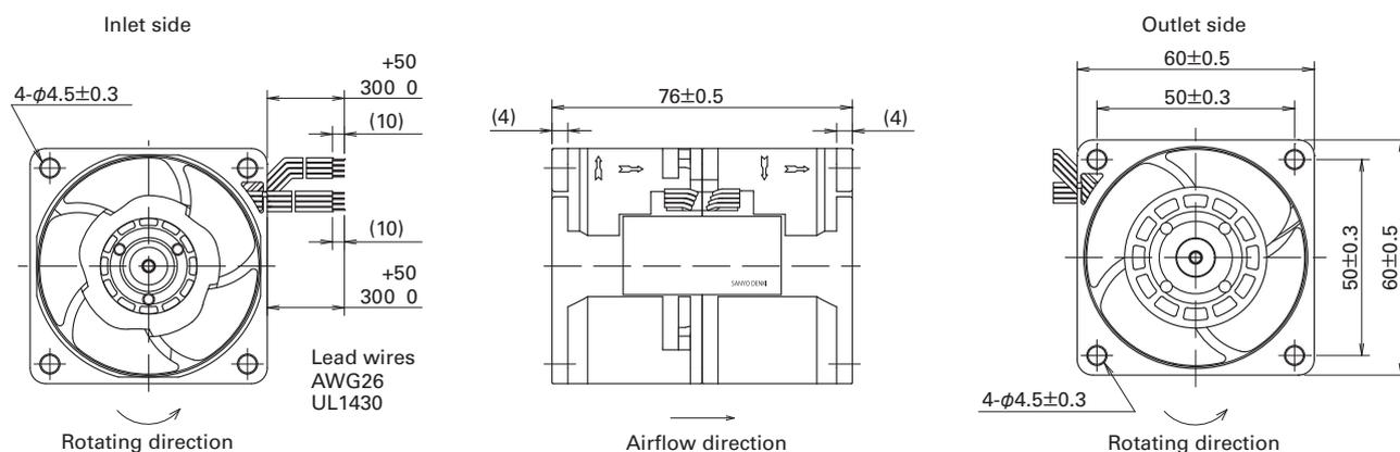
Fig. 2: "San Ace 60" CRA type dimensions (unit: mm)
