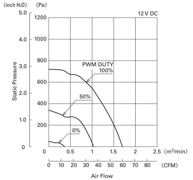
Fig. 6: Air flow vs static pressure characteristics at individual PWM duty cycle(9CRA0612P0S001)
