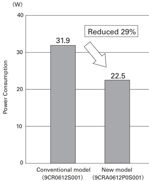
Fig. 9: Comparison of power consumption when operated at presumed system impedance
