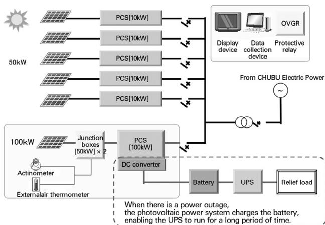
Kangawa Works photovoltaic power system diagram
