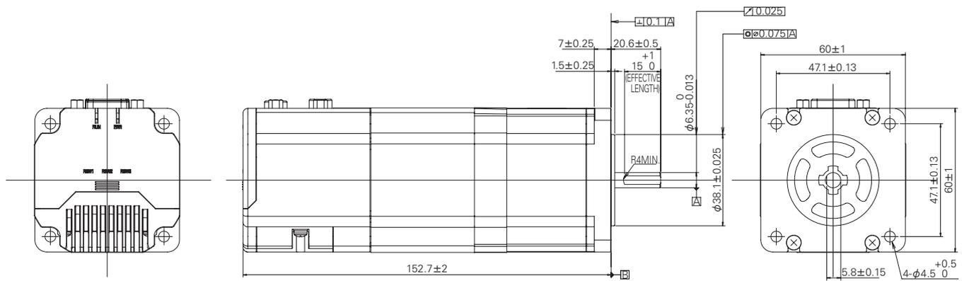
Fig. 6: 60 mm square built-in brake type DPF2M562SB01
