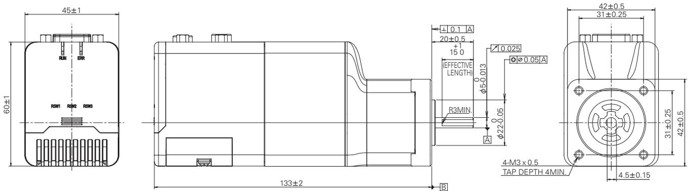
Fig. 4: 42 mm square built-in brake type DPF1M542SB01
