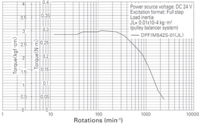
Fig. 7: DPF1M542S-01 torque characteristics
