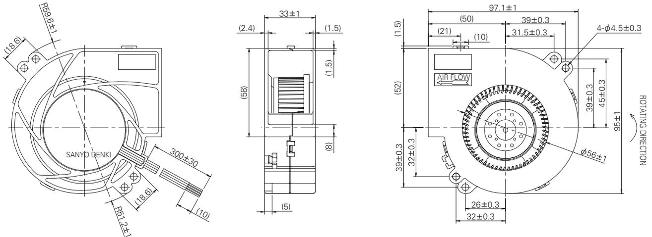
Fig. 2: "San Ace B97" BMB type dimensions (unit: mm)
