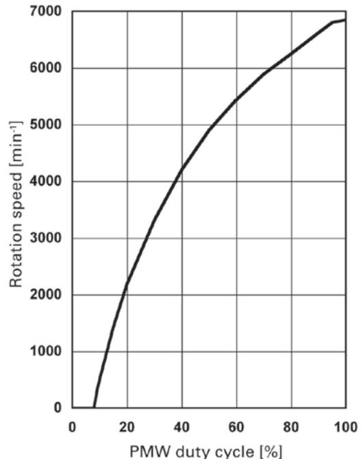
Fig. 4: 9BMB12P2K01 PWM duty cycle and speed characteristics
