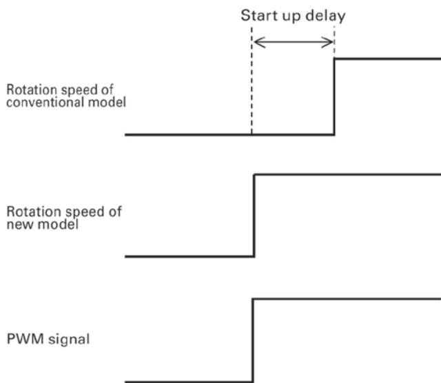
Fig. 8: Scheme of PWM starting signal
