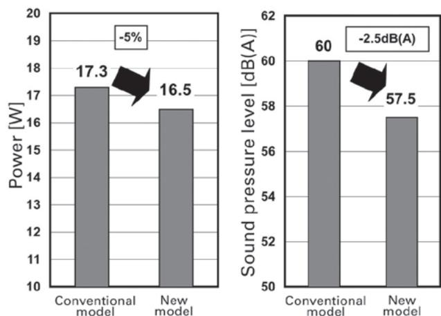
Fig. 7: Power consumption and sound pressure level comparison at operation point A
