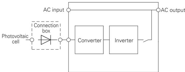
Fig. 6: Power conditioner circuit architecture
