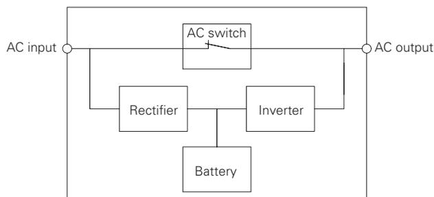
Fig. 2: 3-Mode system (efficiency priority mode)
