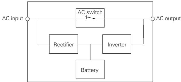
Fig. 2: 3-Mode system (efficiency priority mode)
