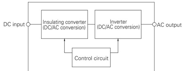
Fig. 8: Circuit architecture of the inverter equipment
