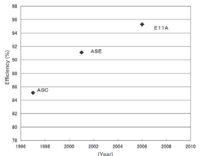
Fig. 1: Efficiency transition of the small capacity UPS
