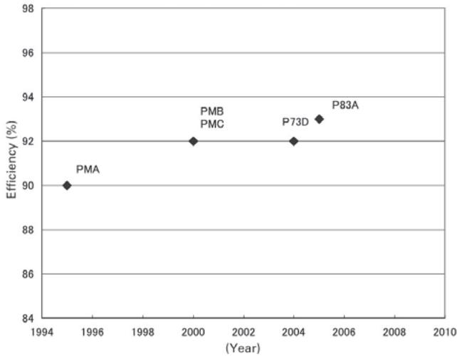
Fig. 5: Efficiency transition of the photovoltaic power generation power conditioner
