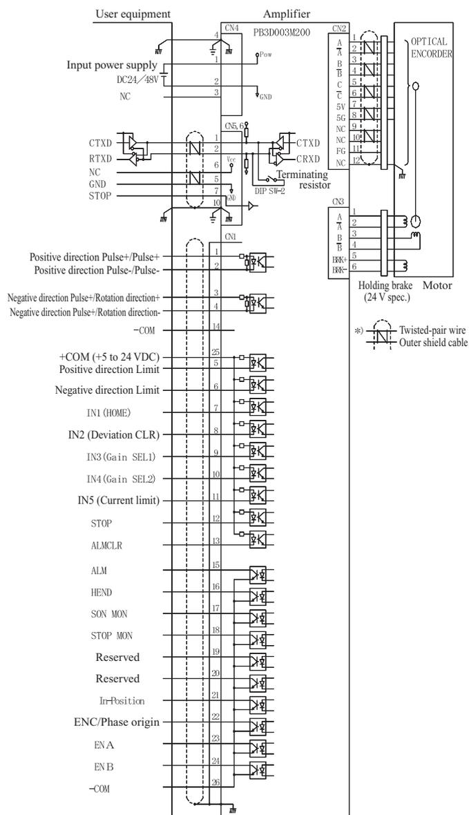
Fig. 3: External wiring diagram for the pulse train interface
