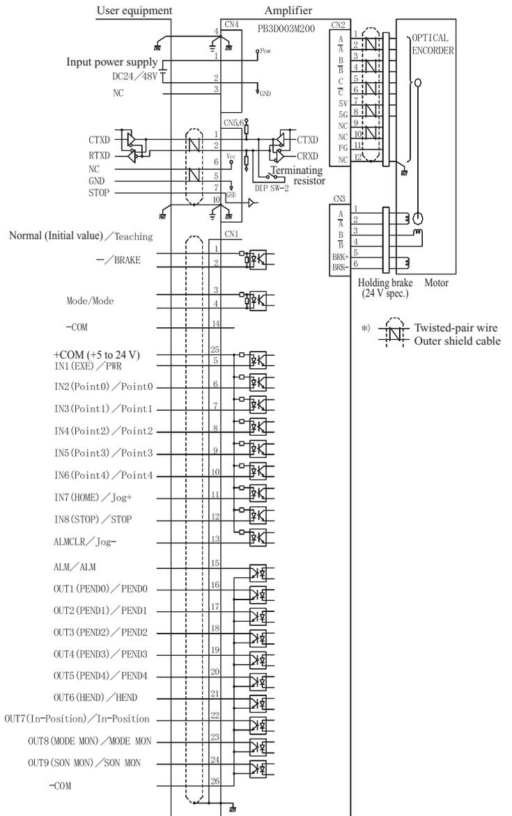
Fig. 2: External wiring diagram for the RS-485 interface
