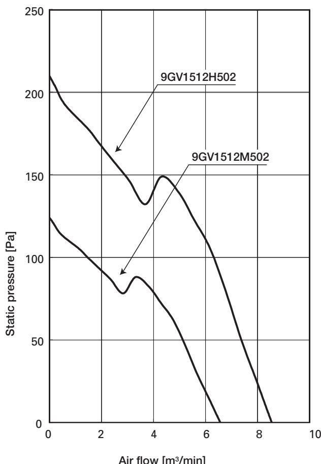
Fig. 3: Air flow vs. static pressure characteristics
