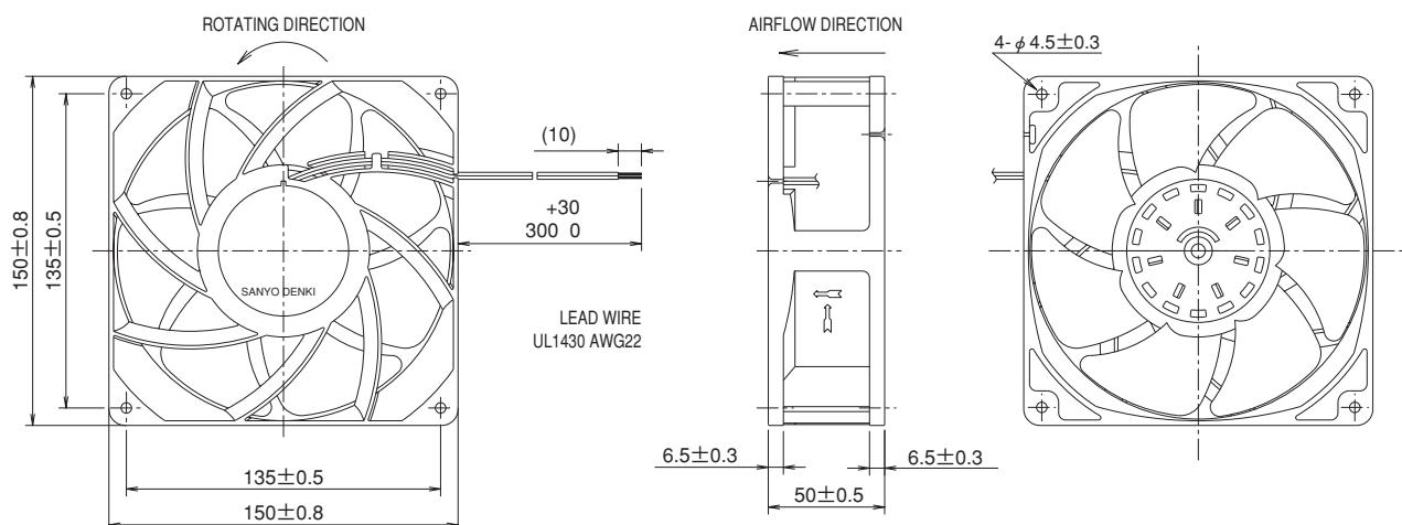
Fig. 2: Dimensions of the "San Ace 150" GV type fan
