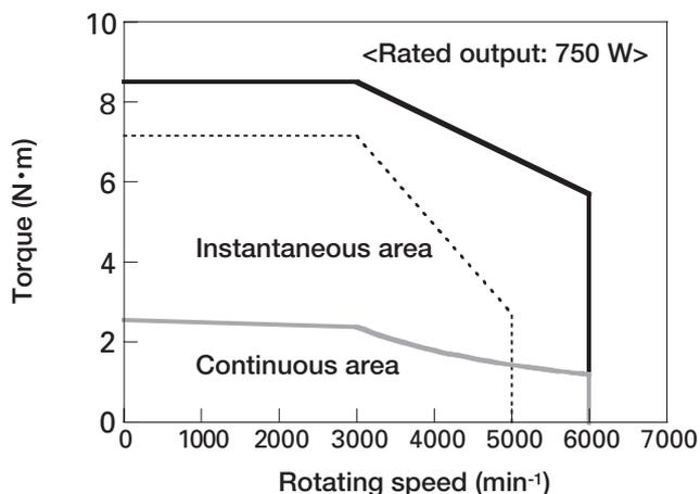
Fig. 9: Torque speed (T-N) characteristics
