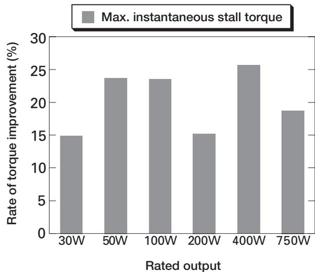
Fig. 6: Rate of improvement for max. instantaneous stall torque (Compared to previous Sanyo Denki models)
