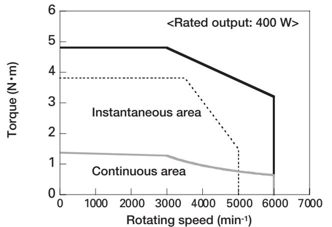
Fig. 7: Torque speed (T-N) characteristics
