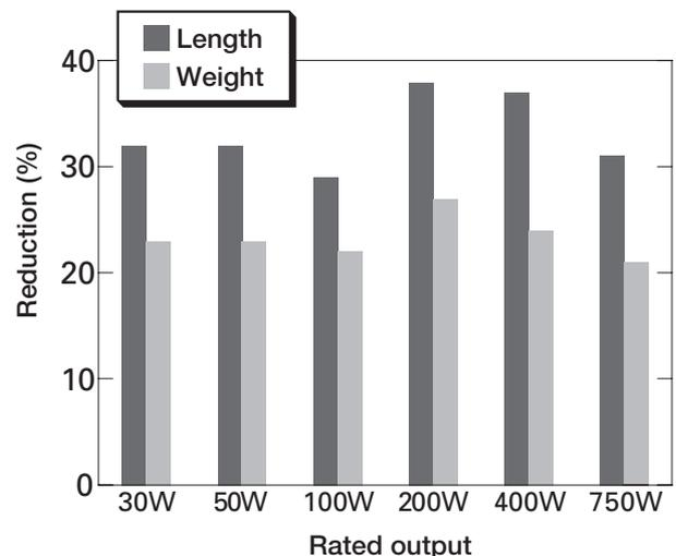
Fig. 2: Reduction in motor length and weight (Compared to previous Sanyo Denki models)
