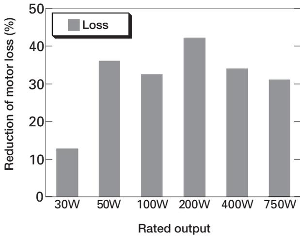
Fig. 4: Reduction of motor loss (Compared to previous Sanyo Denki models)
