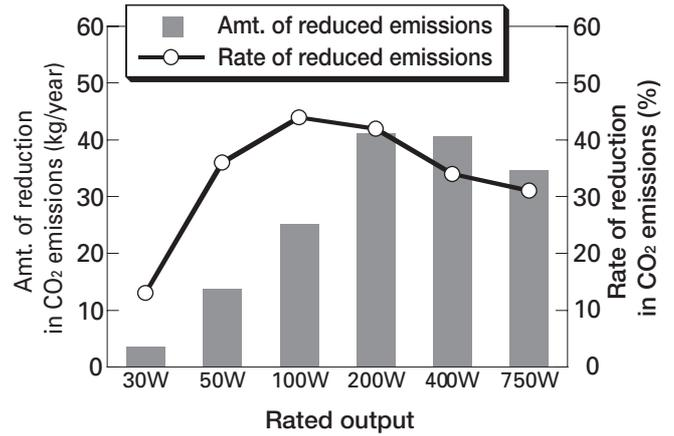
Fig. 5: Rate and amount of reduction in CO<sub>2</sub> emissions (Compared to previous Sanyo Denki models)
