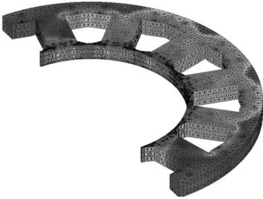
Fig. 3: 3D electromagnetic analysis (1/2 model of the distribution for magnetic flux density of the stator core)
