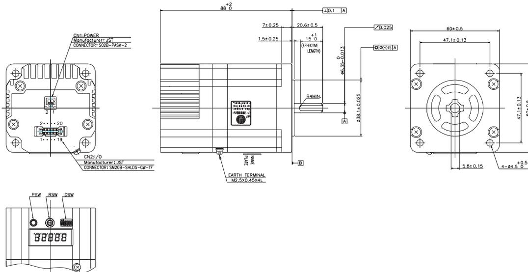
Figure 3 Exterior view of the 60 mm sq. DB22M162S-01
