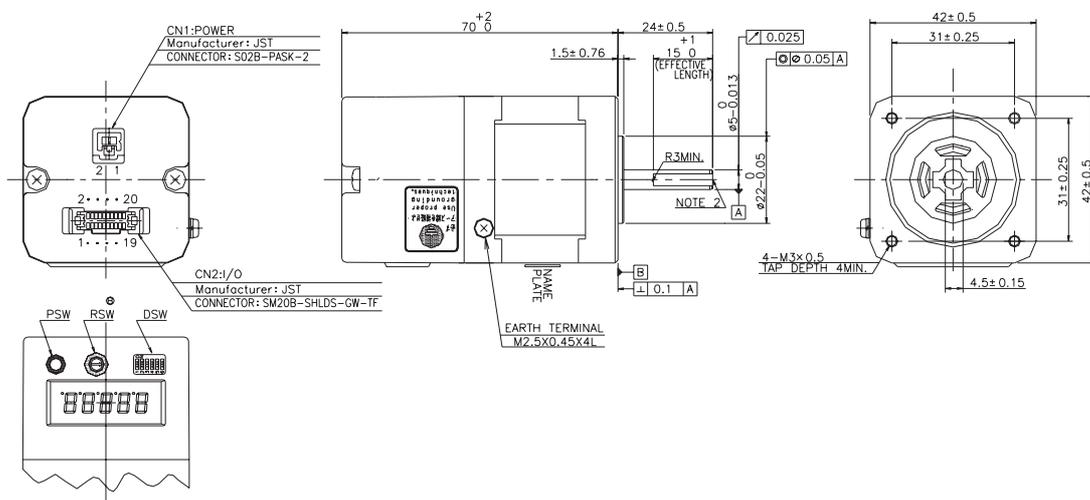
Figure 2 Exterior view of the 42 mm sq. DB21M142S-01
