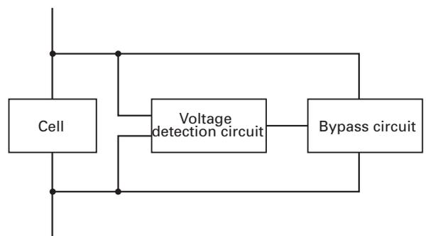
Figure 5.1 Bypass system
