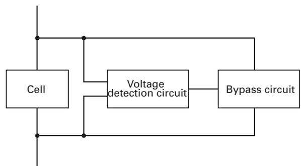
Figure 5.1 Bypass system
