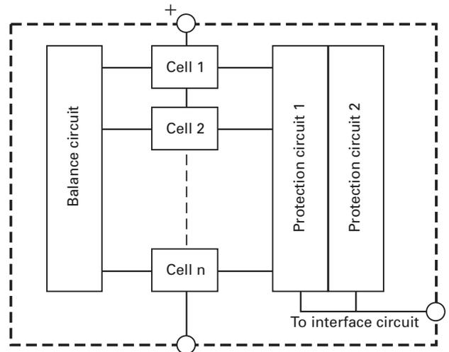
Figure 4 Basic layout of battery module
