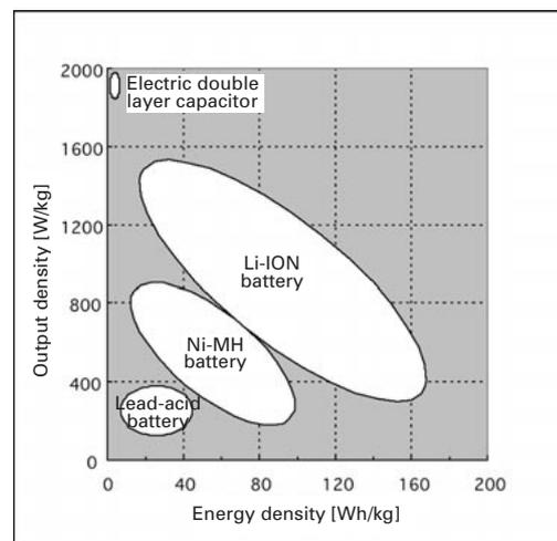
Energy density: the amount of electrical power the unit can produce in one hour
