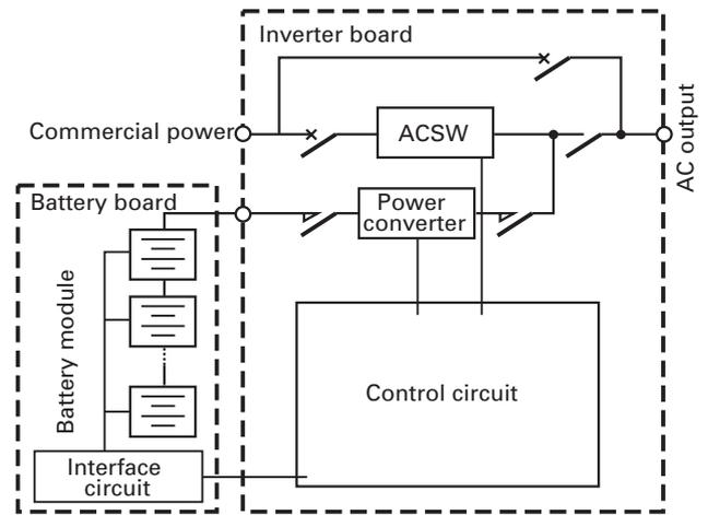
Figure 3 Basic layout of “SANUPS E23A-Li”
