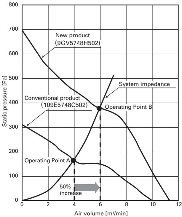
Figure 4 Comparison of air volume vs. static pressure characteristics
