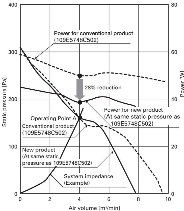
Figure 5 Comparison of air volume vs. static pressure characteristics and power consumption characteristics
