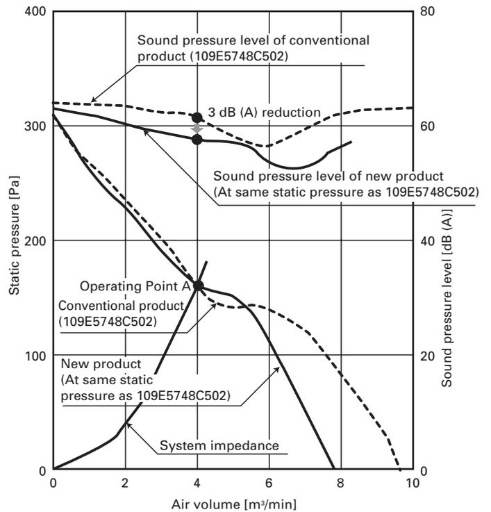
Figure 6 Comparison of air volume vs. static pressure characteristics and sound pressure characteristics
