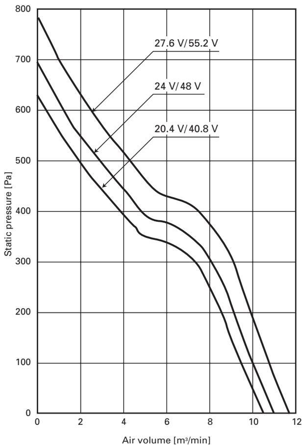
Figure 3 Air volume vs. static pressure characteristics
