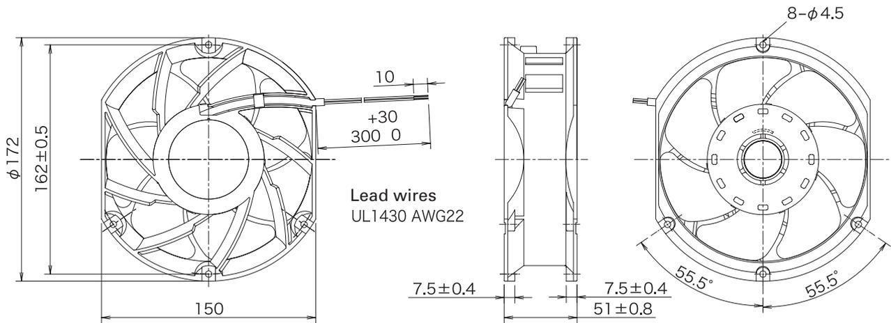
Figure 2 Dimensions of the "San Ace 172" GV type fan
