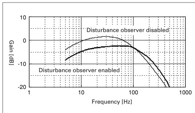
Fig. 4 Disturbance suppression characteristics
