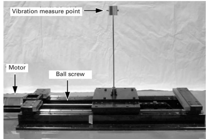
Fig. 5 Damping control evaluation machine
