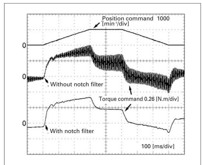
Fig. 3 High-frequency resonance suppression characteristics
