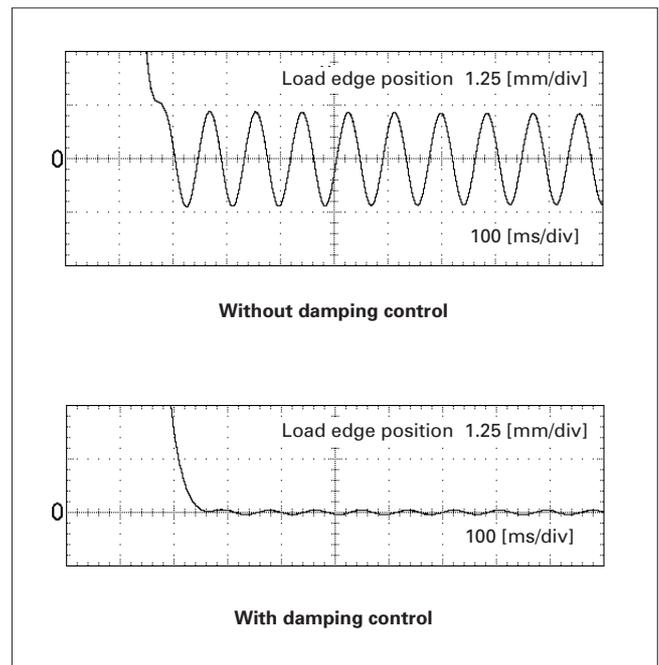
Fig. 6 Damping control characteristics
