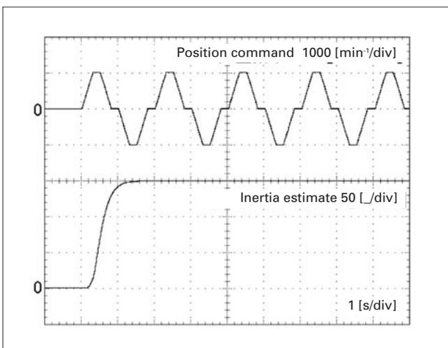
Fig. 2 Inertia estimation characteristics
