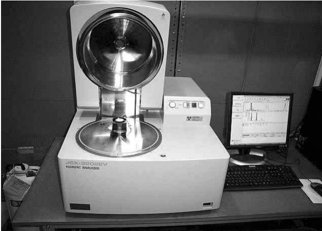
Fig. 4 Energy dispersive X-ray fluorescence analyzer (EDXRF)
