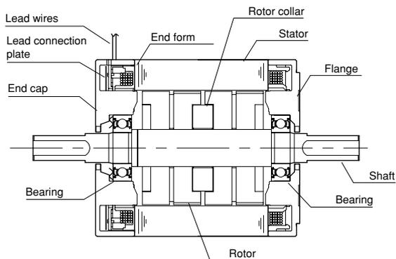
Fig. 3: Structure of the Motor
