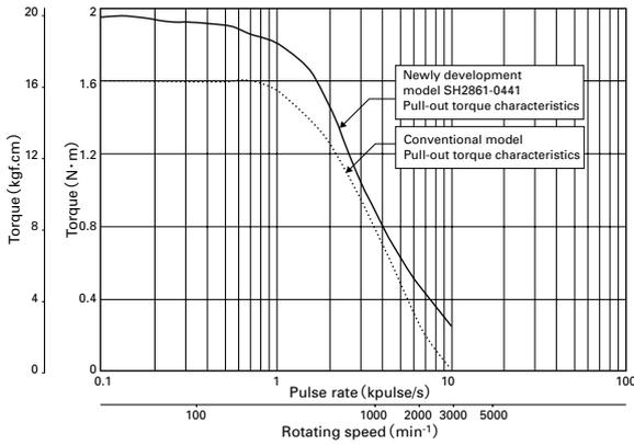
Fig. 5: Comparison of Pulse rate – Torque Characteristics for SH2861-0441/ 0411
