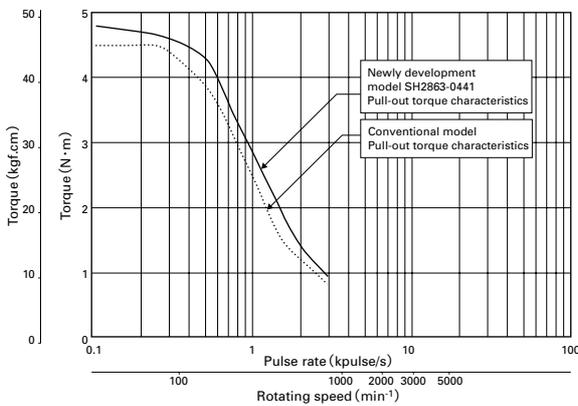
Fig. 7: Comparison of Pulse rate – Torque Characteristics for SH2863-0441/ 0411
