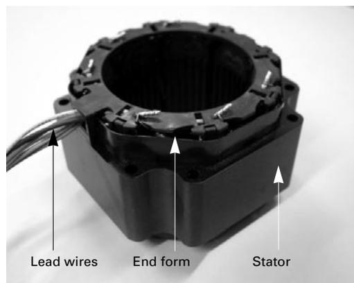
Fig. 4: Inside the Motor
