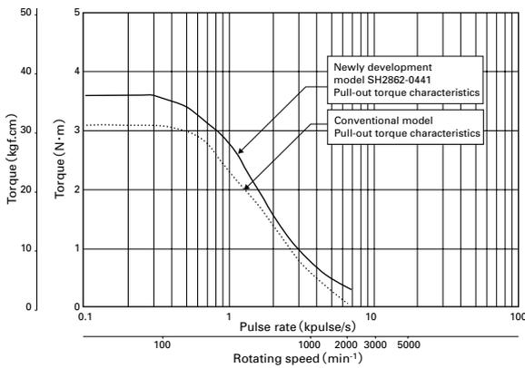
Fig. 6: Comparison of Pulse rate – Torque Characteristics for SH2862-0441/ 0411
