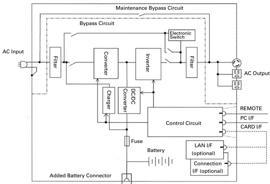
Fig. 4: Circuit Block Diagram
