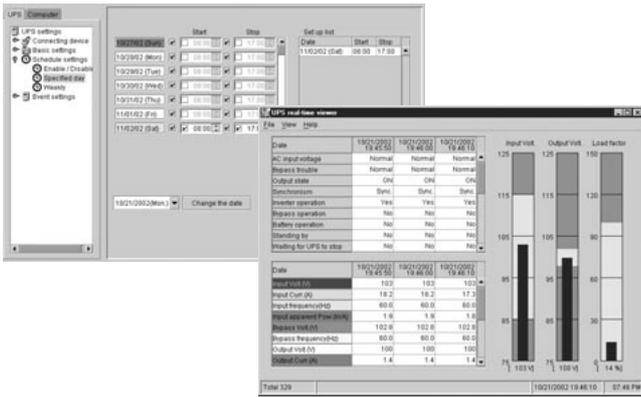
Fig. 3: Screen Shots from Power Supply Management Software
