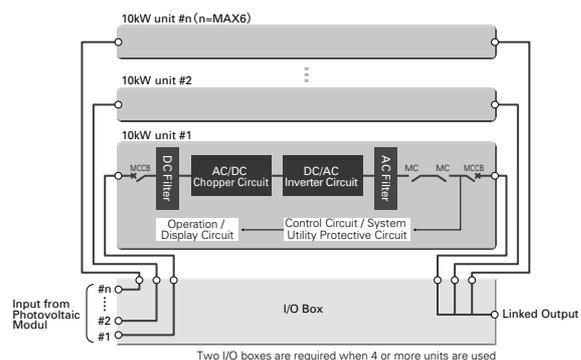
Fig. 3: Circuit System Block of "SANUPS P73E"
