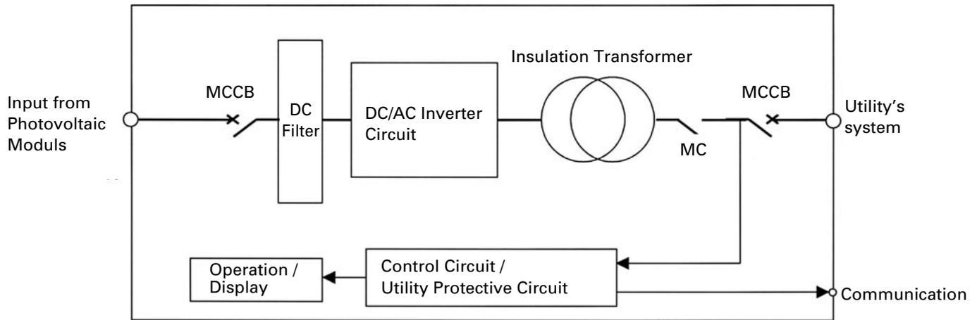
Fig. 2: Block Diagram of the "SANUPS P83A"
