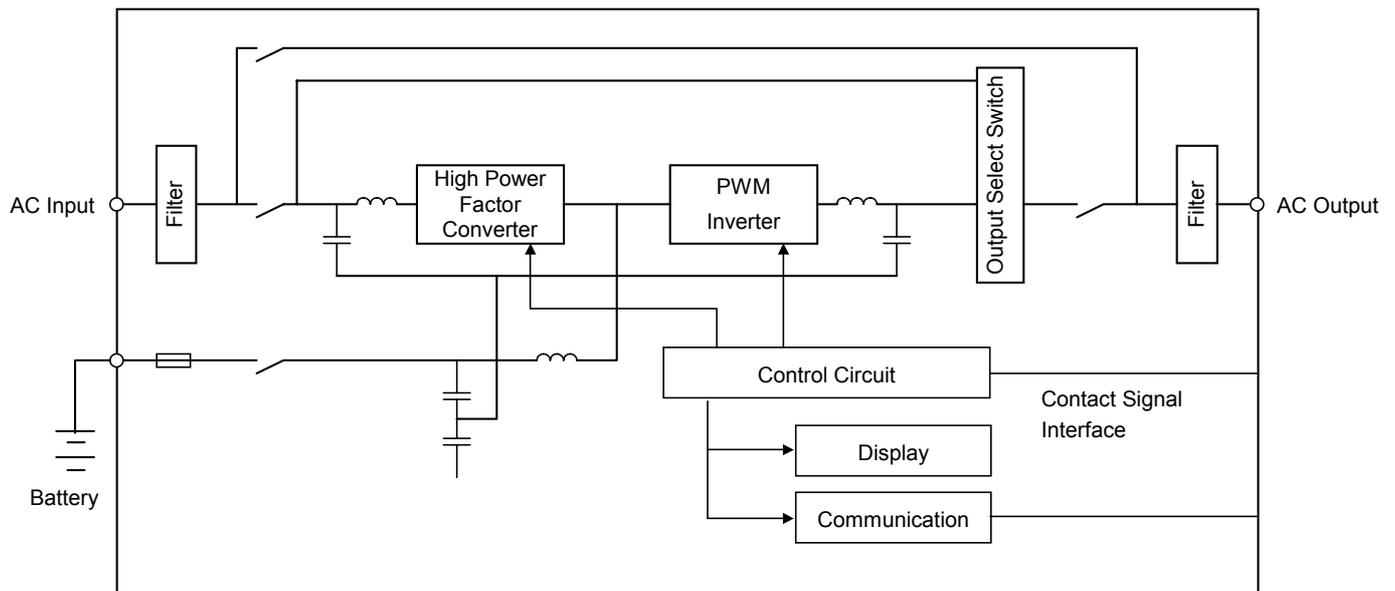
Fig. 2 Circuit Block "SANUPS" A23C
