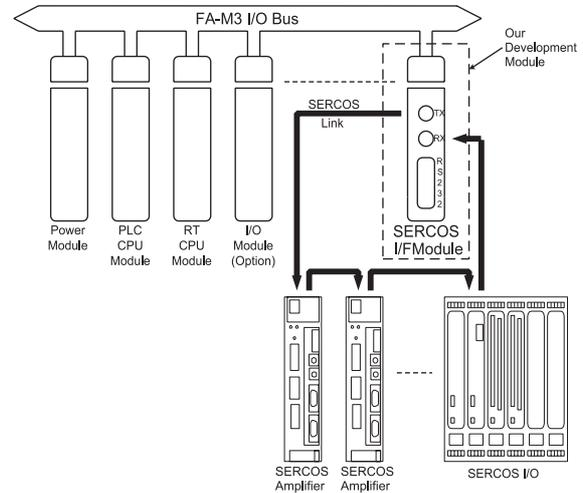
Fig. 1 Configuration Diagram of FA-M3
