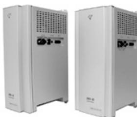
As part of the "S-MAC PC" series of industrial PCs, the "SMS-10", which uses an Am486DX-133MHz as a CPU and a PC/104 bus as an internal bus, has already been released. However, these days, some user applications require the high-throughput CPUs. Demand is also high for 32-bit PCI bus. To propose solutions to meet these demands, we developed the "SMS-30".
