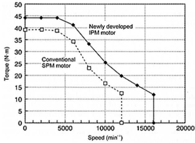
Fig. 2 Torque speed characteristics
