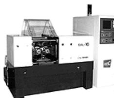
The unit controls five servo motors and one hydraulic servo, and consists of a complex system for full close and torque feedback. It has been jointly developed with a machine maker by sharing expertise and experiences. This control system has thus become the object of many patents applied for and the company is proud of it on an international level.
