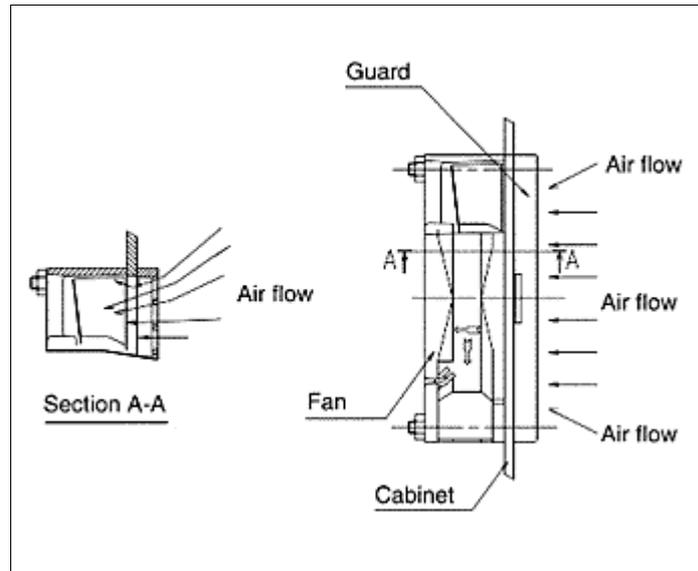
fig. 9 Air Flow in a traditional product on the market, as equipped with a resin Finger guard
