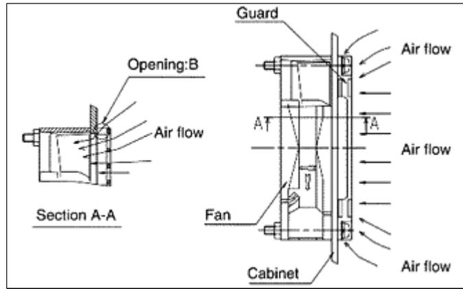
fig. 8 Air flow in the new product as equipped with a resin Finger guard
