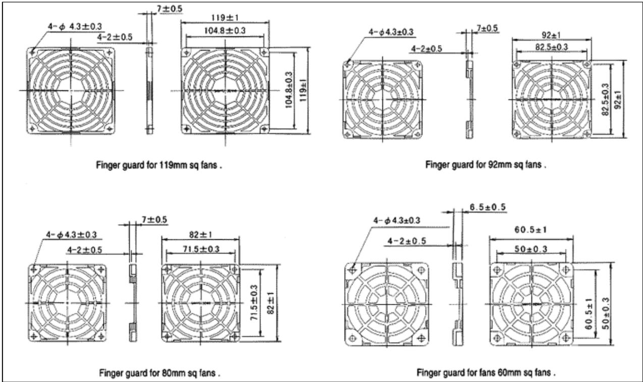
fig. 11 Outside dimensions of resin Finger guards
