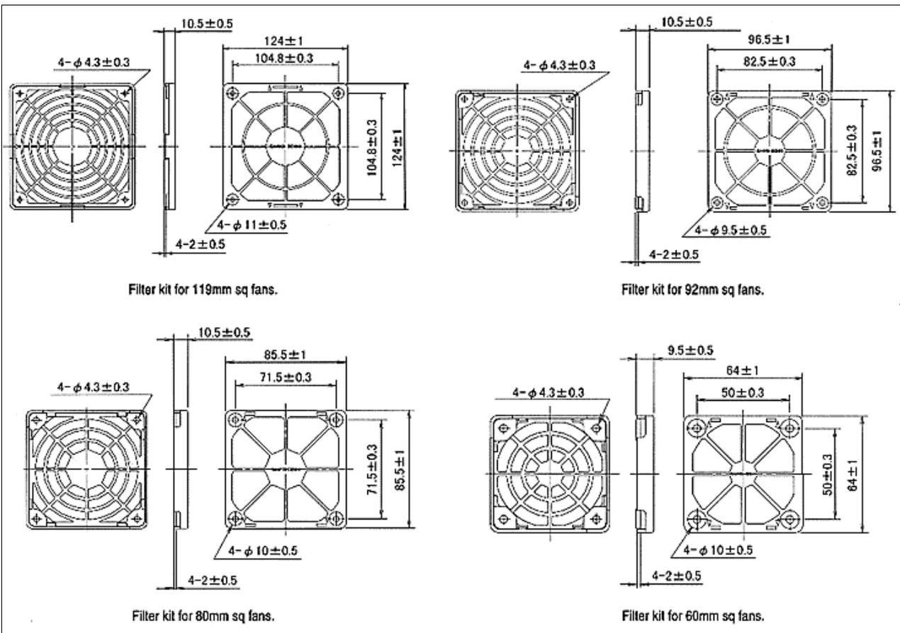
fig. 5 Outside dimensions of Filter kits
