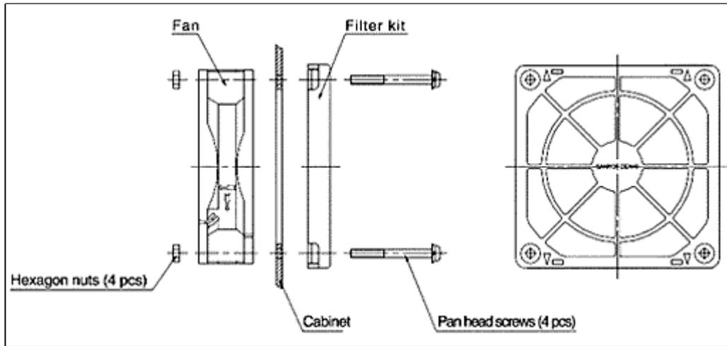
fig. 4 How to install the new product
