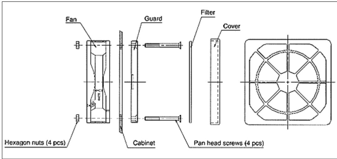
fig. 3 How to install traditional models
