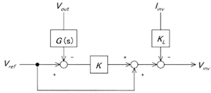
Fig. 11 Proposed control circuit
