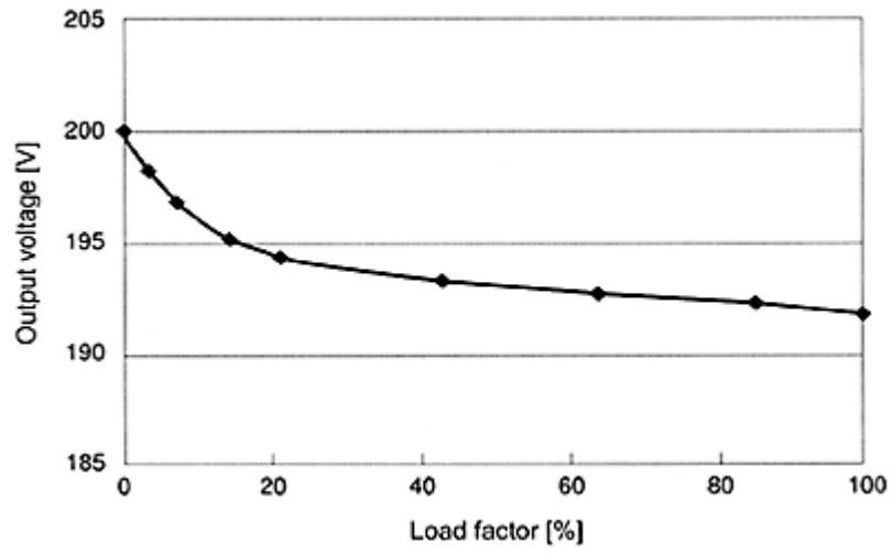
Fig. 8 Output voltage with regard to load factor
