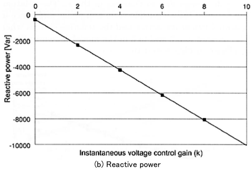
Fig. 7 Active and reactive powers of the cross current with regard to the gain
