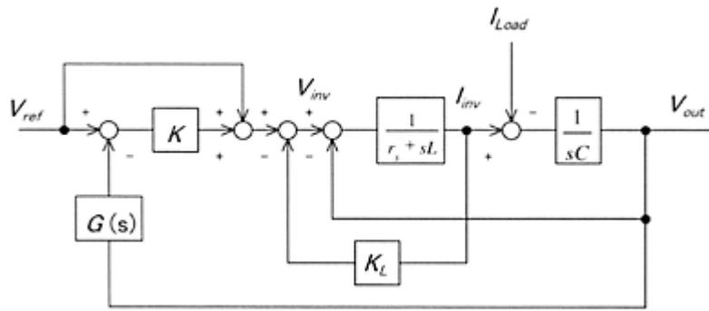
Fig. 12 Block diagram of parallel run control of UPS
