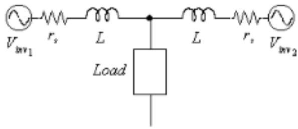
Fig. 1 Parallel connected model of UPS
