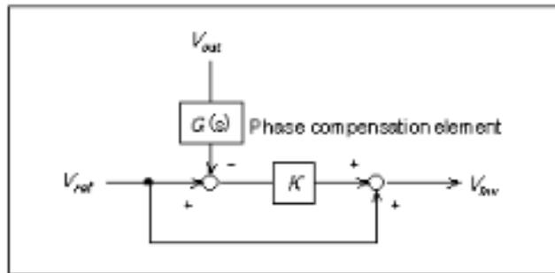
Fig. 4 Block diagram of inverter control
