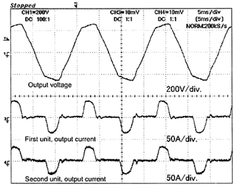
Fig. 14 Experimental results (when the rectifier is loaded)
