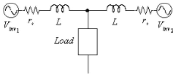
Fig. 1 Parallel connected model of UPS
