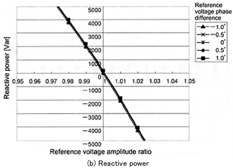
Fig. 6 Active and reactive powers of the cross current with regard to voltage ratio and amplitude difference
