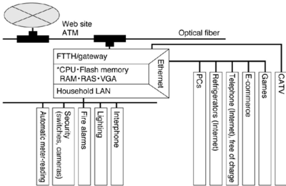
Fig. 9 A typical implementation of the " SMS-10 " as an FTTH gateway
