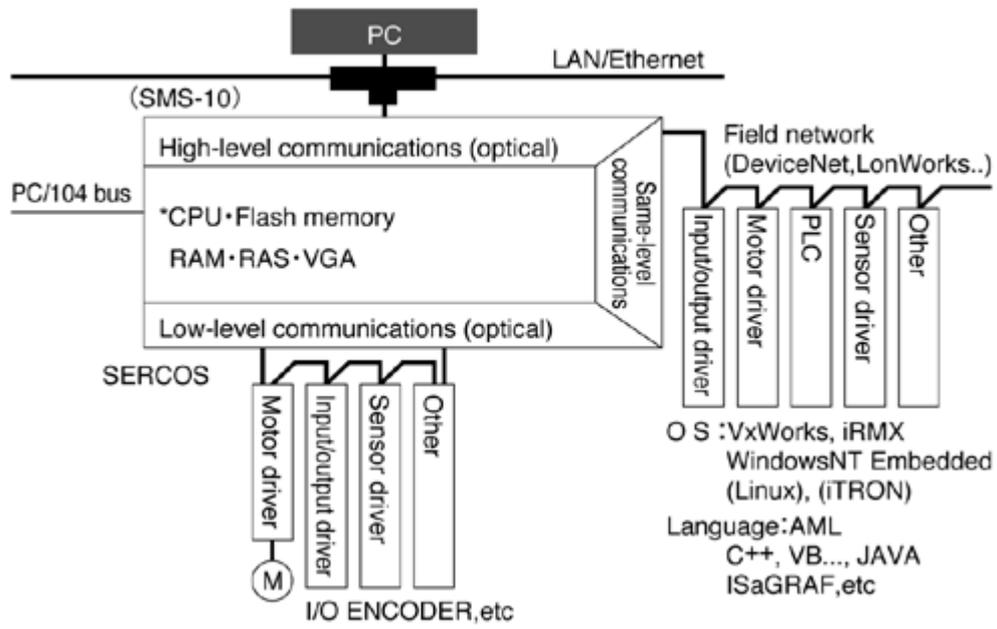
Fig. 8 Interface configuration of " SMS-10 "
