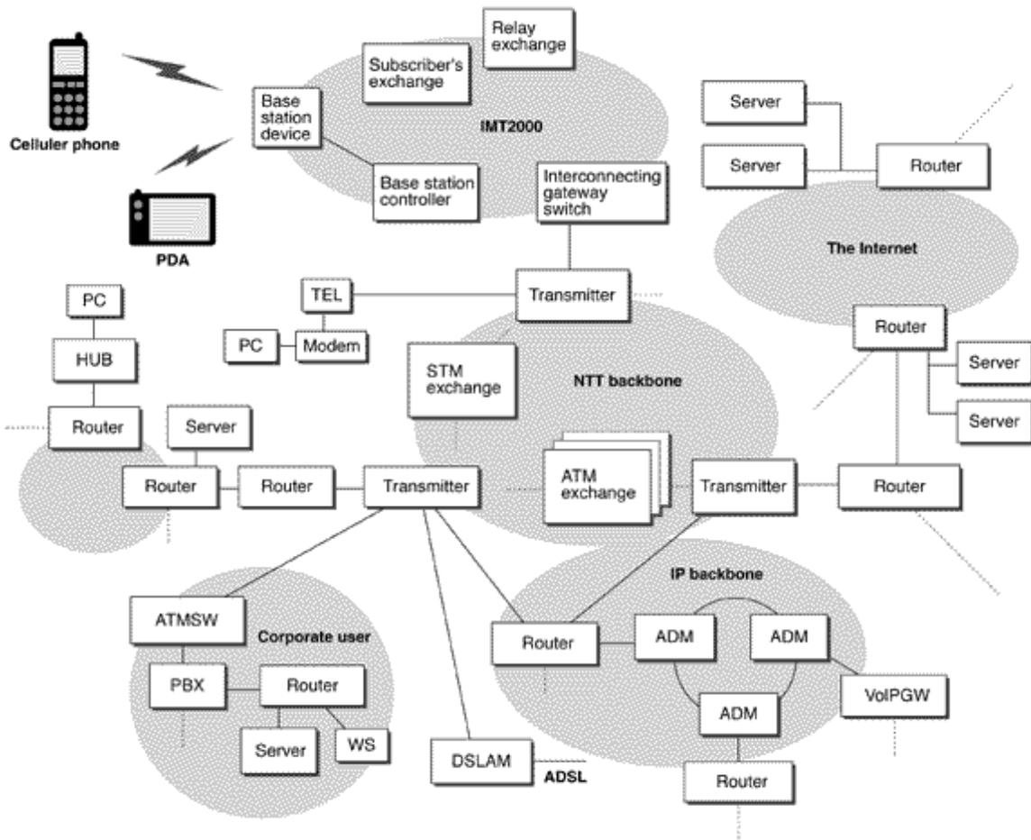
Fig. 3 Image chart of a typical communications network
