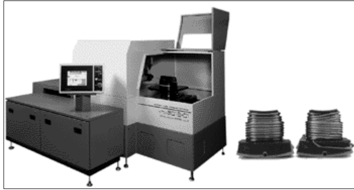
fig. 14 Outside view and fabricated samples of wire winding machine
