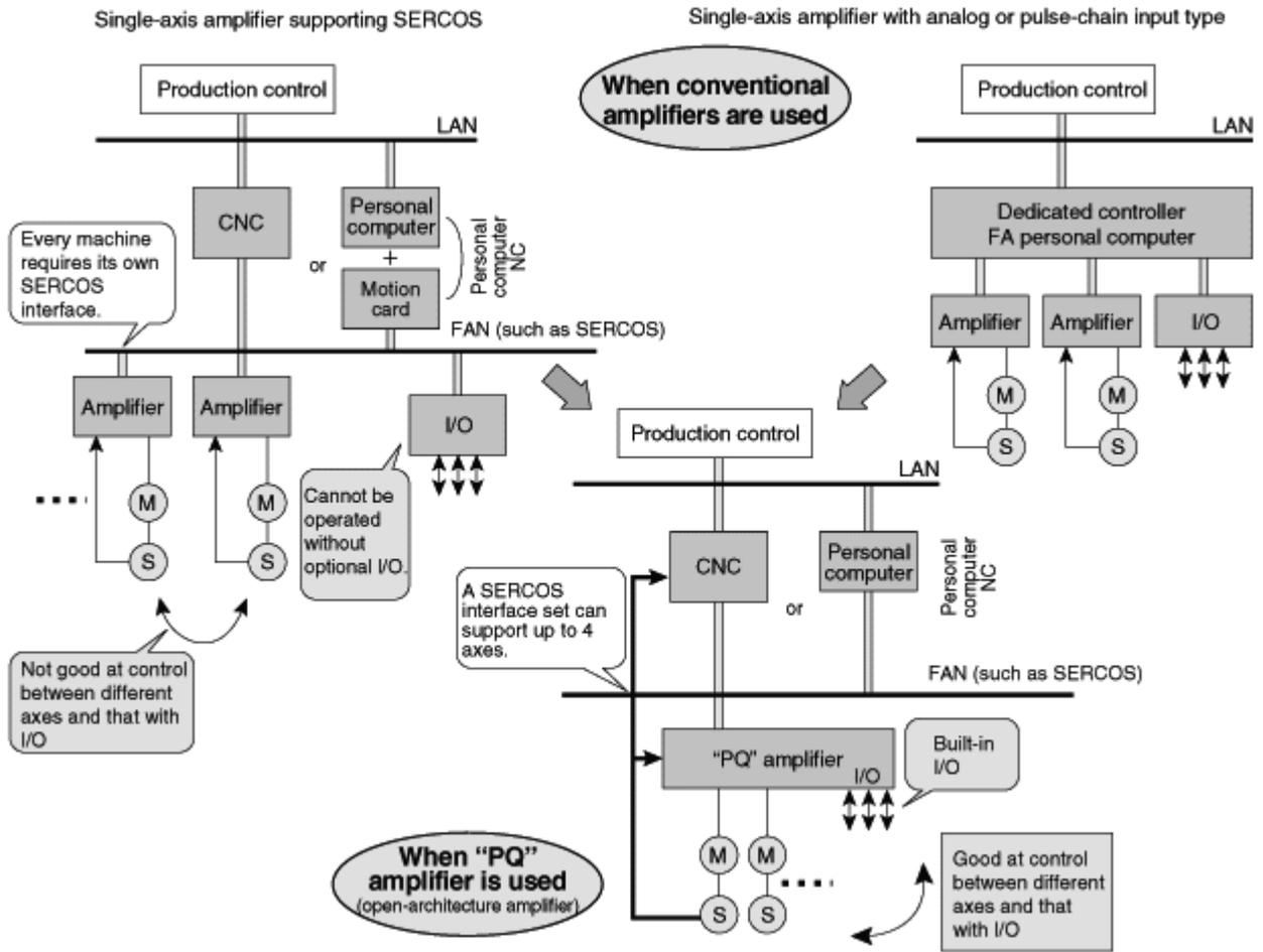
Fig. 2 Comparison of configurations between conventional type amplifier and PQ amplifier
