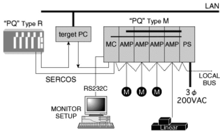
**Fig. 1 Example of "PQ" configuration**
